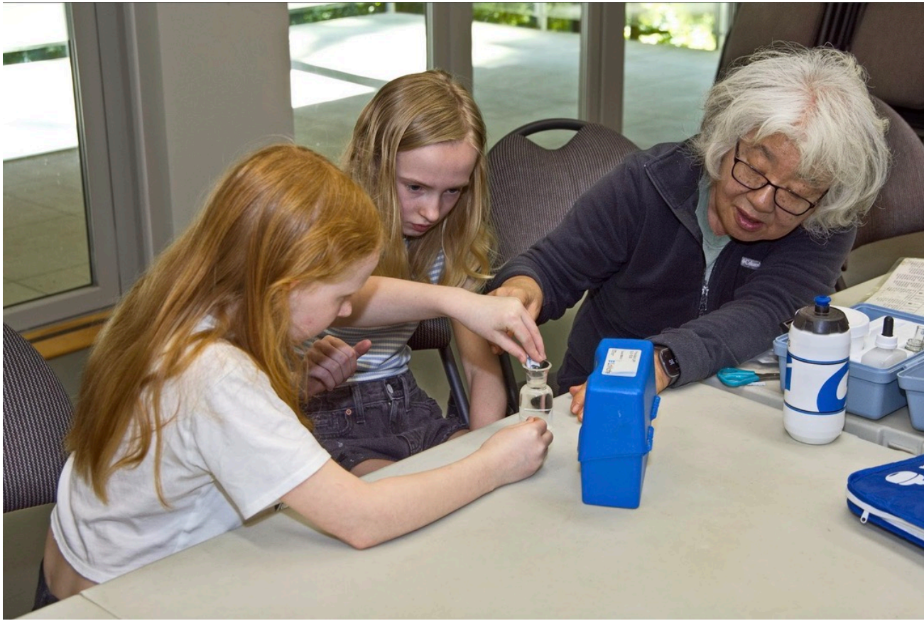
Addy and June assist with measuring O_2 using the Hach titration method.
